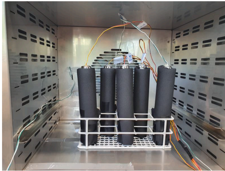
Fig. 3. Samples inside the climate chamber.
